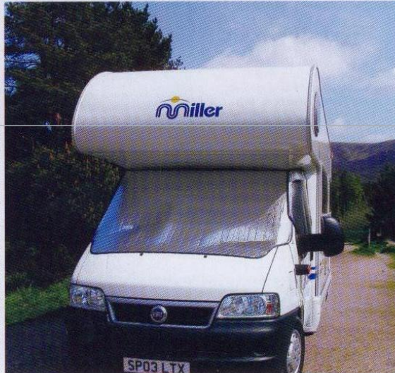
The external windscreen cover sheds any water clear of the upper bonnet edge.
