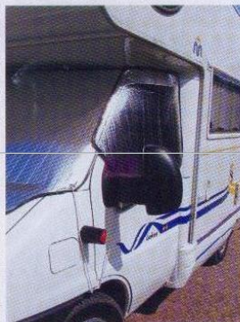
Attachment of external screens includes bungee cord to the wheel arch.
