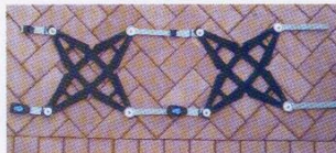
Two of the three sections that link together to fit on each wheel.
